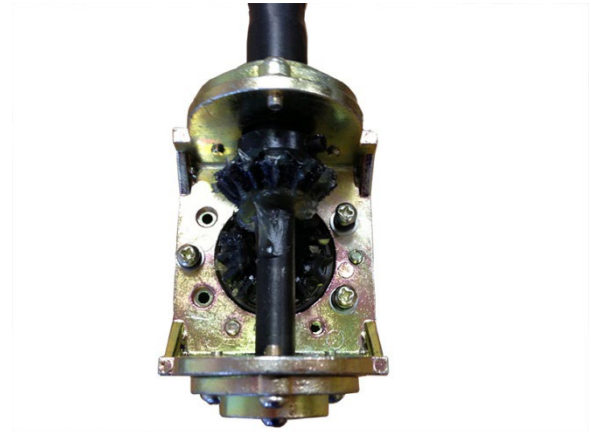
Figure 24. Umbrella Gear without the cover.
