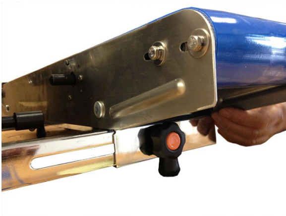
Figure 19. Remove the two knobs underneath the conveyor to slide the conveyor off the conveyor support.
