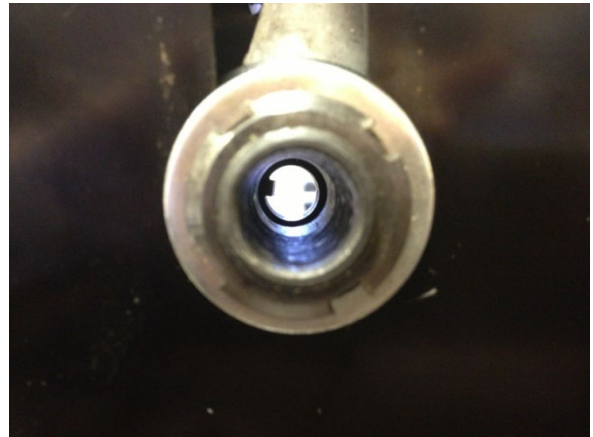
Figure 28. Take note of the alignment groove in the axis hole.
