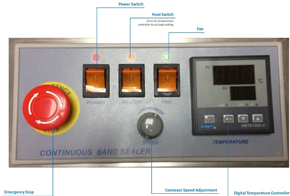
Figure 9. Control Panel of CBS-880
